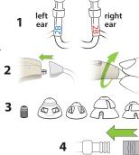
4 Align tip with end of sound tube and push tip straight on
